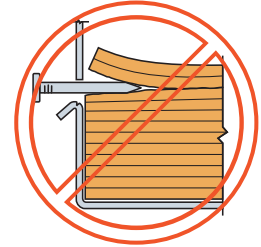
Nail at Wrong Angle
